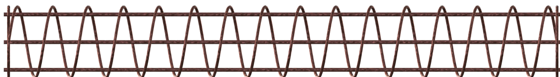
2083071CSLM x 1 SL WIRE ROPE REINFORCING CAGE 2325L RQUIRED FOR PILE FOUNDATION ONLY
