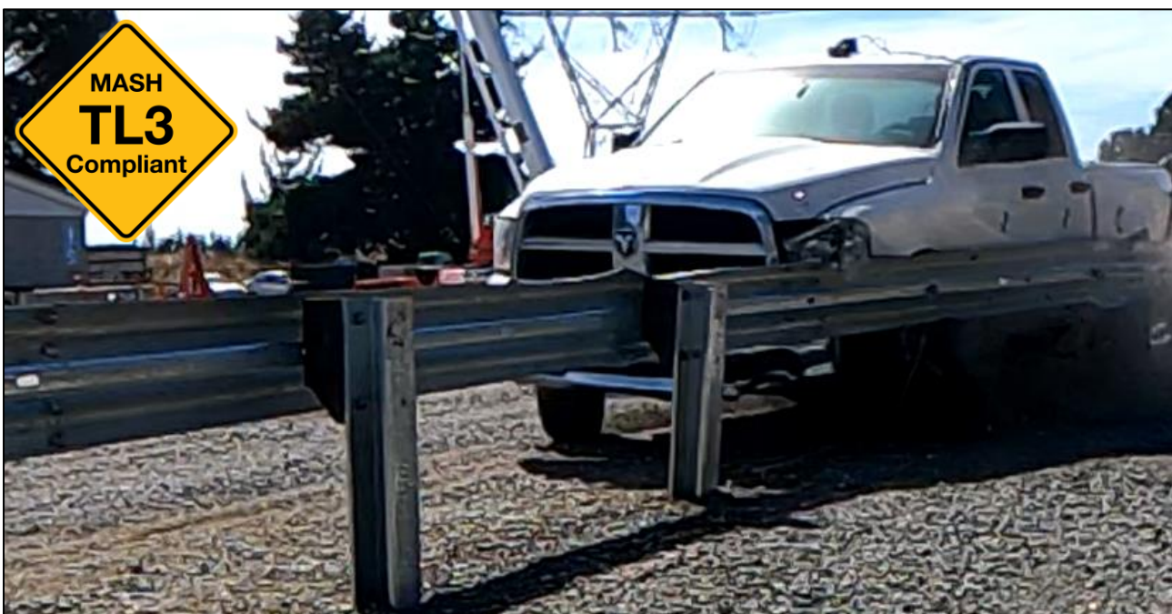
Figure 1: Full-Scale Crash Testing of RamShield® Low Deflection with RamBlocs®.
