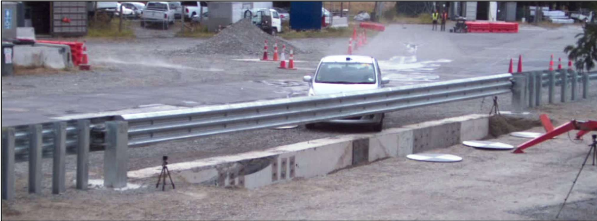
Figure 1: Crash Test Impact: 1100kg Passenger Car, 100km/h and 25 degrees
