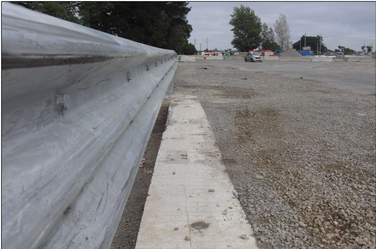
Figure 8: Nil Damage to CrocGuard® Following MASH 4-10 Impact
