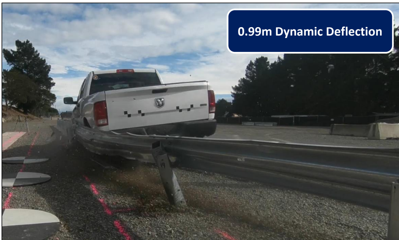
Figure 2: G4 W-Beam with RocketBloc™, MASH TL3 Containment & Redirection
