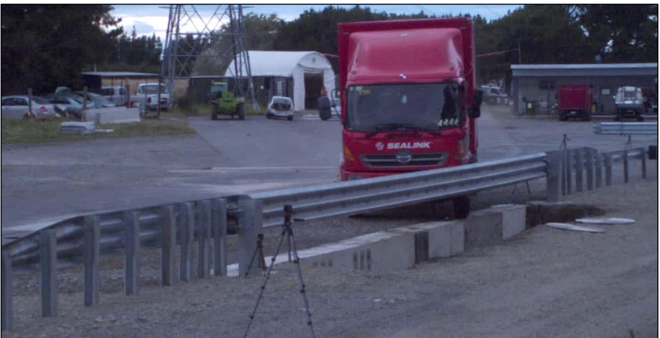
Figure 3: Crash Test Impact: 10,000kg Rigid Truck, 90km/h and 15 degrees
