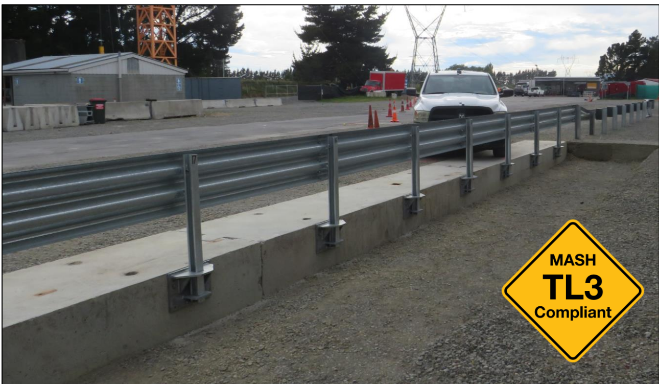
Figure 3: Crash Test Assessment of HammerBeam™ on the Edge of an Elevated Concrete Beam.
