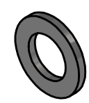
VFX164 M16 Flat Washer Form 'C' (34 O/D x 3.0mm Thick) (VG001166) 0.01 Kgs [0.02 lbs]
